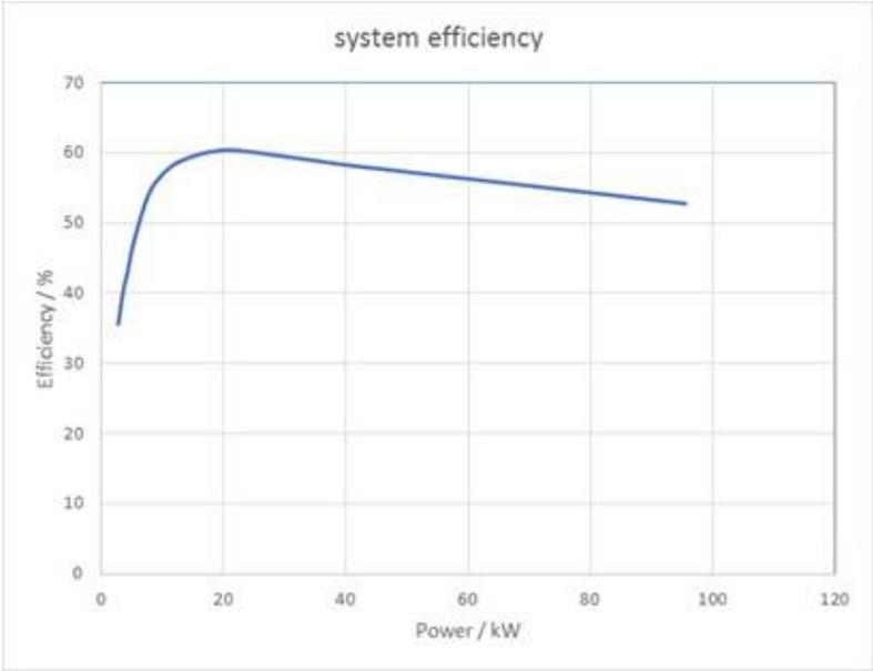
Figure 39: Graph displaying the fuel system cell efficiency as a function of power output.
